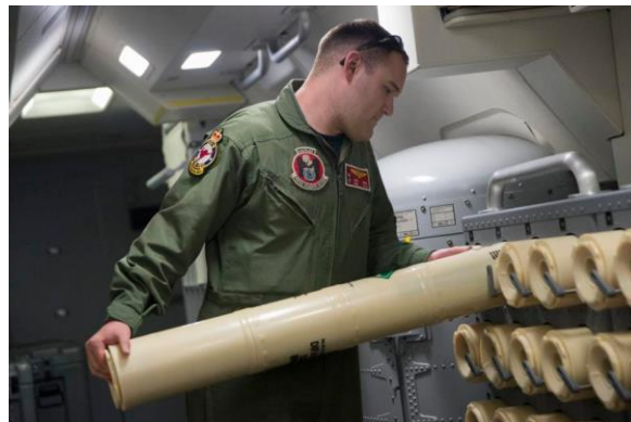
Figure H-4: Loading a Sonobuoy in a P-8 Poseidon Aircraft
