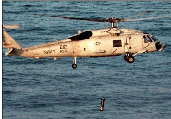
Figure H-5: Helicopter Deploys Dipping Sonar
